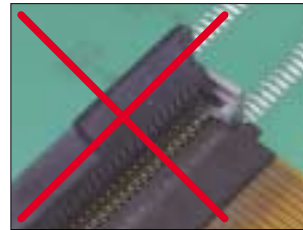
Incorrect FPC insertion
