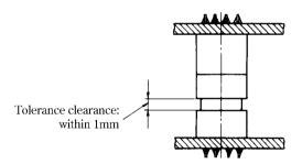
Set the tolerance clearance within 1mm to mate the male and female connectors. (Except for the lock cable type)
